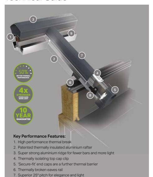
8. Adjustable reinforced stopper to prevent glass slipping9. Choice of aluminium or uPVC internal and external cappings
